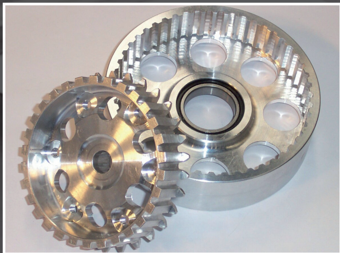
Custom made lightweight aluminium clutch assembly
