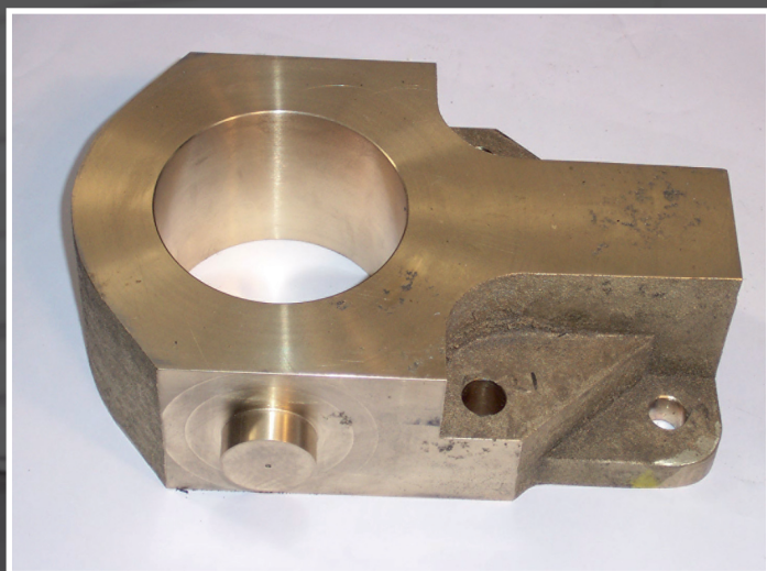
Bronze and aluminium steering gear components
