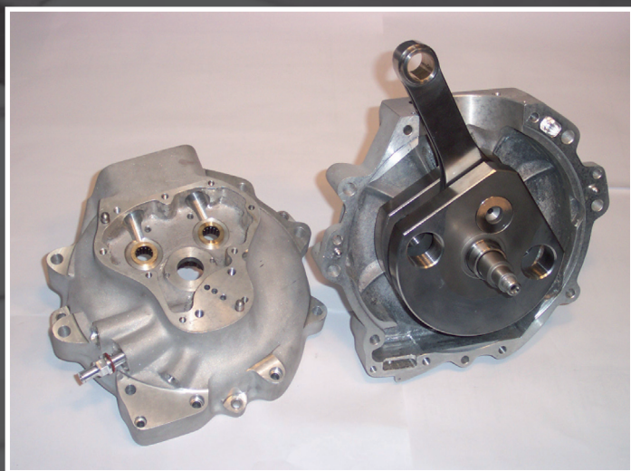
Purpose built short stroke single cylinder motorcycle engine
